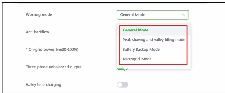
The energy storage inverter provides four working modes to meet the needs of users in different applications, namely
