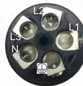
Figure 3-37 Connecting an AC output power cable (4)
